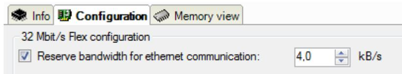
Figure 48: Reserving bandwidth for Ethernet communication.
