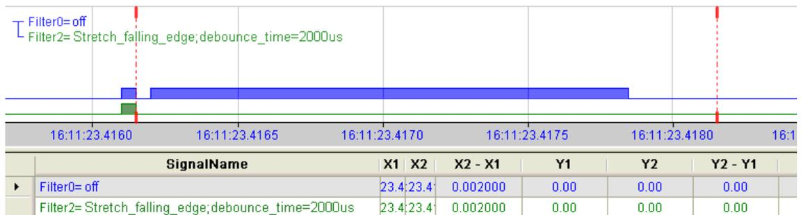
Figure 8: Debounce filter: "Stretch falling edge"
