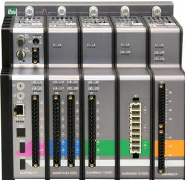
The iba modular system acquires and processes measurement signals and, with the appropriate signal output modules, is perfectly suited for control applications. The decisive advantage of the system is the freely configurable concept: a central unit can be combined with up to four additional input/output modules.
